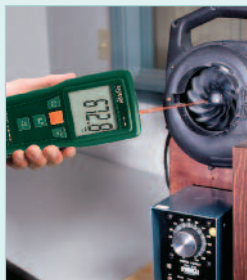
Photo Tachometer function measures the speed of rotating objects without contacting the surface by using a laser beam and reflective tape
